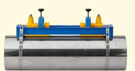
Xonic 100GC is a transit-time ultrasonic flowmeter with outstanding performance compared to the differential pressure flowmeter. Depending on pipe size, system use 1 or 2 path ultrasonic sensor and use temperature sensor for volume compensation. Xonic 100GC is the first clamp-on ultrasonic gas flowmeter developed in Korea to replace highend foreign brands by maintaining performance and reducing price of conventional gas flowmeter.
